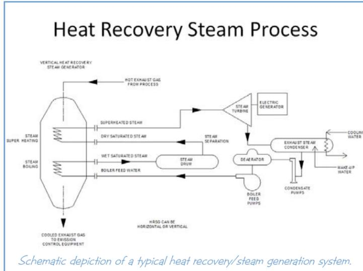
devices has left only minimal room for new equipment. The resulting space constraints will require the steam turbine generator to be on an elevated platform with the condenser hanging below. The heat recovery boilers will be of a vertical design, also due to space constraints. A partial turbine bypass for supplemental process steam is also included.
