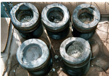
Siloxane deposits on engine pistons
